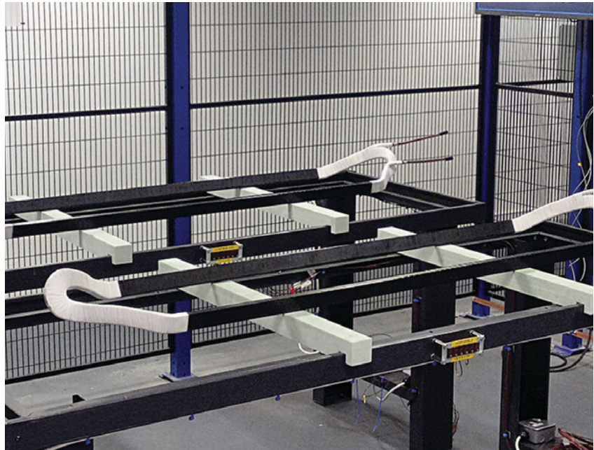
The new coil test lab enables both thermal cycling and voltage endurance testing to be completed in-house.
