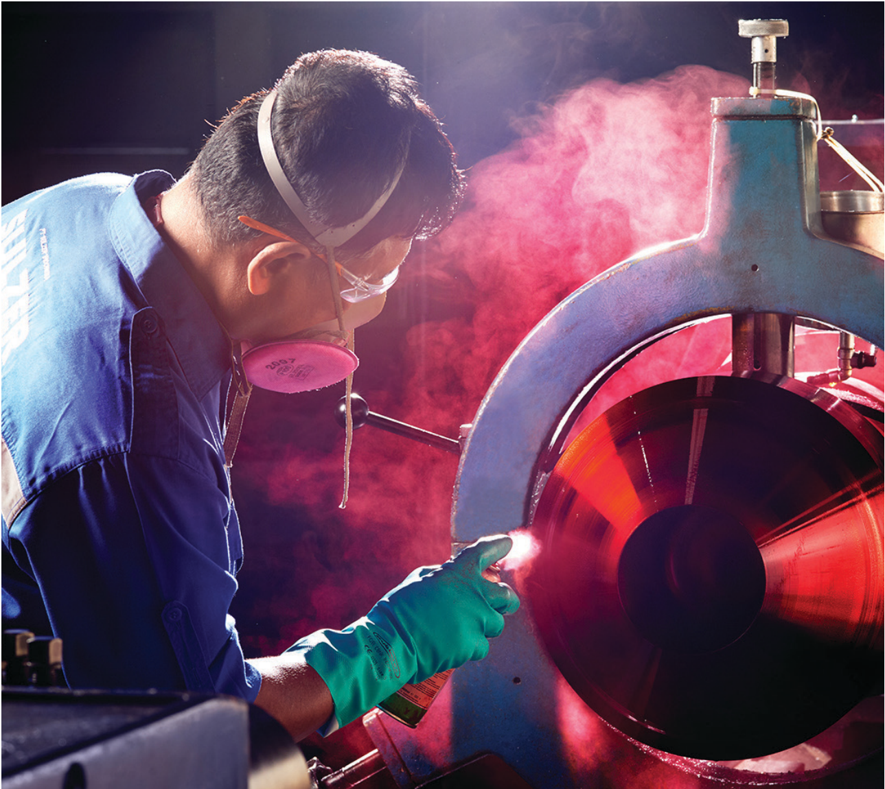
Dye penetrant testing was completed to ensure the new rotor had no flaws
