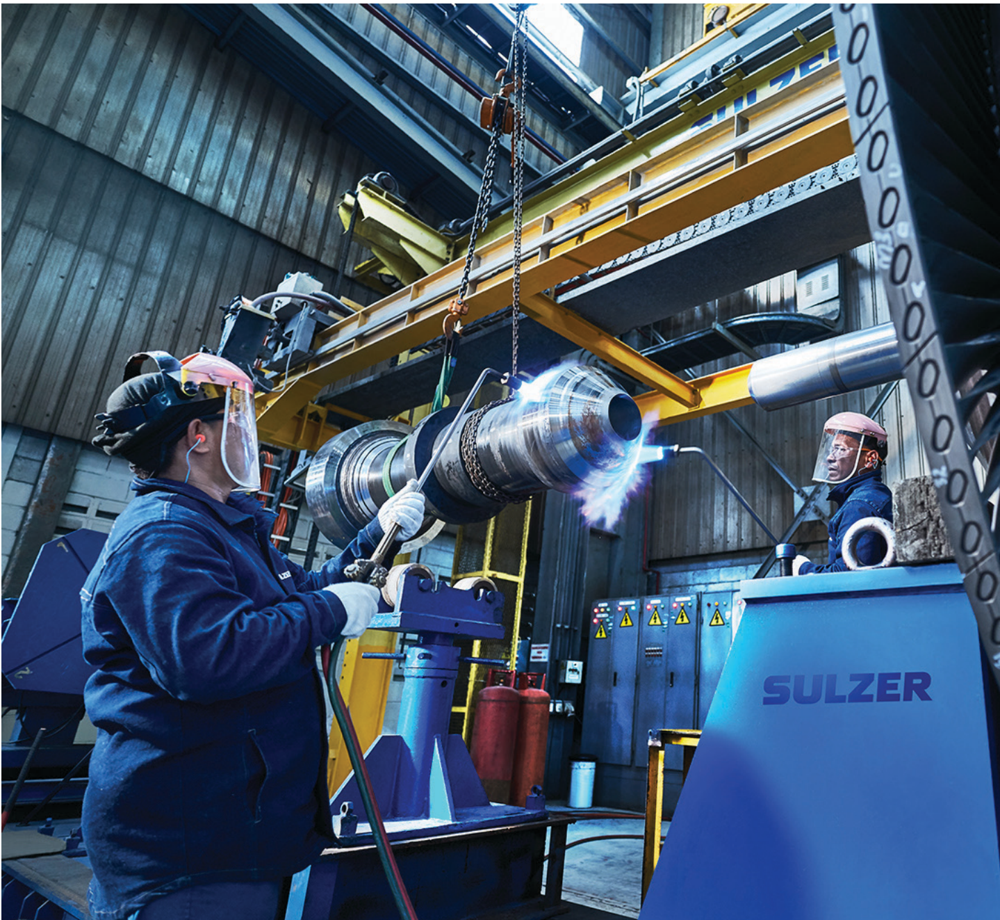
The stub shaft was shrink-fitted to the shaft before being welded in place.
