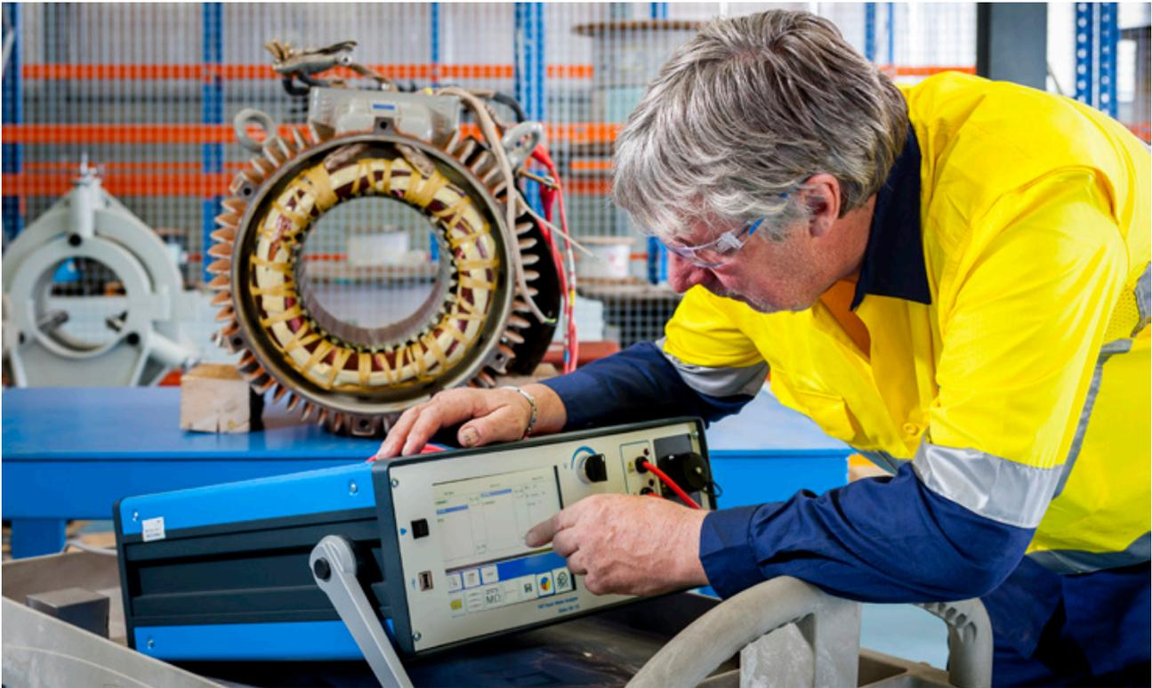
Electrical testing after rewind - credit Sulzer.
