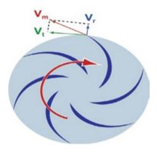
To understand how impeller design affects efficiency, focus on how the pumpage exits the impeller, relative to the angle of the impeller vane at that point. The pumpage is swirling around in the impeller housing outside of the impeller, but at a slower speed of the impeller, but at a slower speed than the tip of the impeller vane. The pumpage is being directed through the impeller and out of the impeller by the impeller vane.
