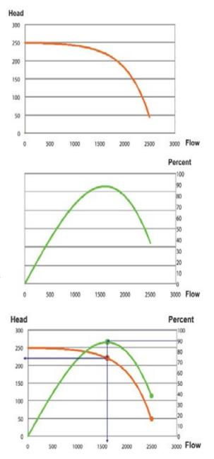
So somewhere between dead head and run out condition, there is a flow rate at which the efficiency is maximum that's the BEP. Note that the BEP is indicated in Figure 3 at a flow rate of about 1600 units; that flow rate coincided with the maximum value on the efficiency curve. That flow rate also intersects the pump curve at a point equal to head of about 220 units.
