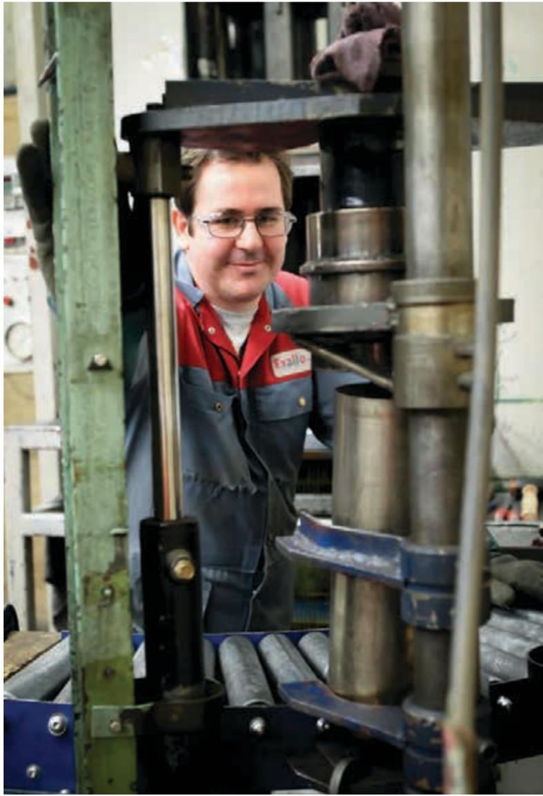
Manufacturing shaft sleeves to protect pump shafts.
