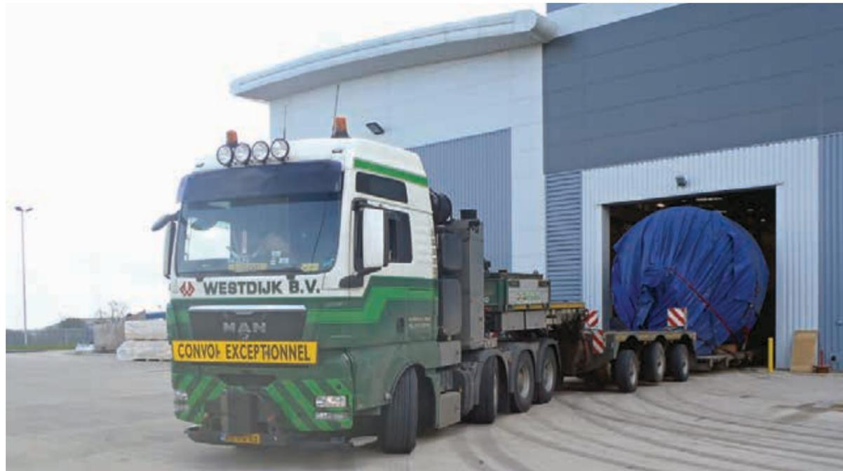
Delivering a 7 metre long, 4 metre diameter, 68 tonne armature for testing at Quartzelec Rugby - special transport permits were required for the transit through Europe and the UK
