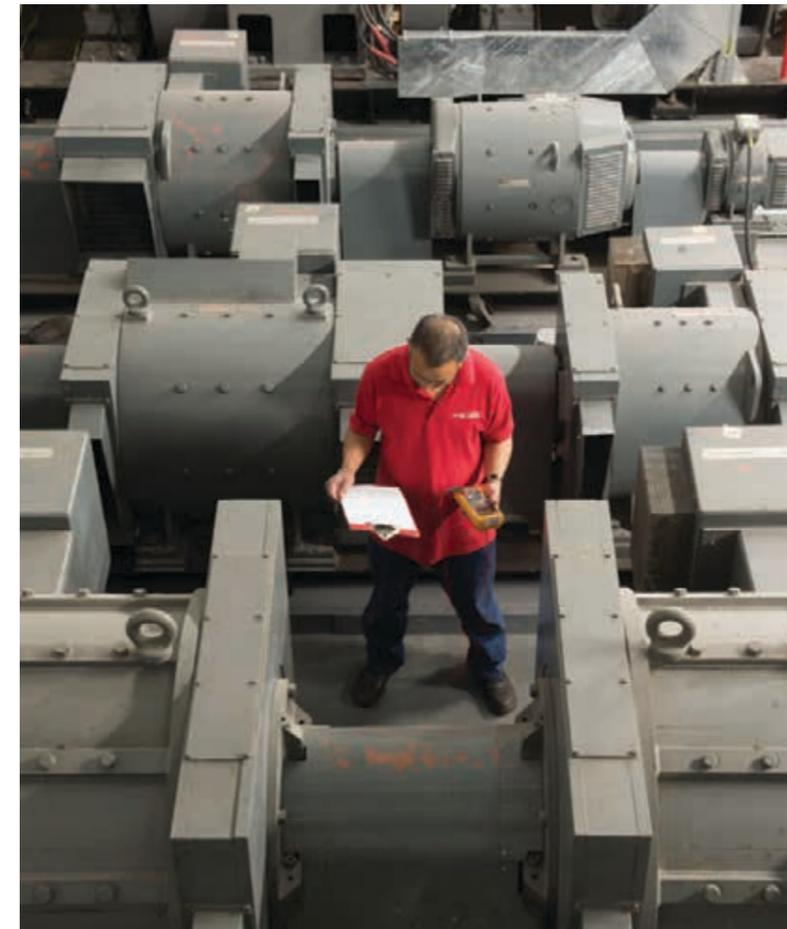
Extensive range of capabilities for testing a wide variety of machines; a sound proofed control room with a state of the art control system and [pictured] the extensive test facility's machine room fed from a 500Vdc 12-pulse rectifier on an 11kV grid supply.
