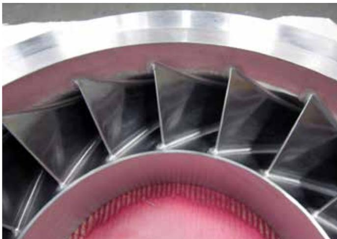
*Modifications to the vane geometry would ensure the optimum inlet flow angle which would also improve the mass flow rate (MFR).*
