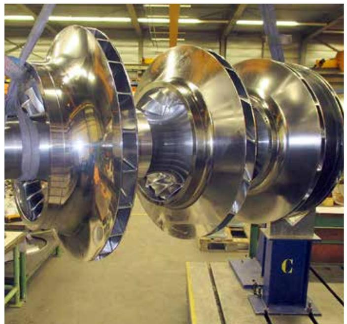
Each impeller was spin tested before being mounted onto the new rotor shaft to ensure the integrity of the impeller construction when operating under load
