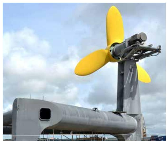
Gravity mounted, direct seawater cooled generator
