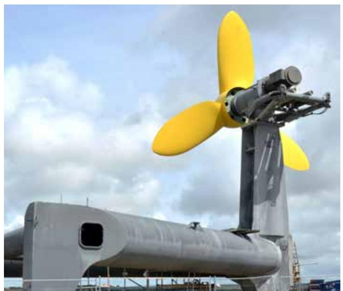
Gravity mounted, direct seawater cooled generator
